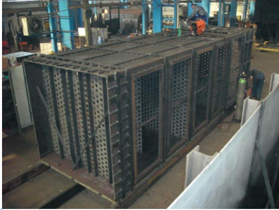
Incineration air preheater
