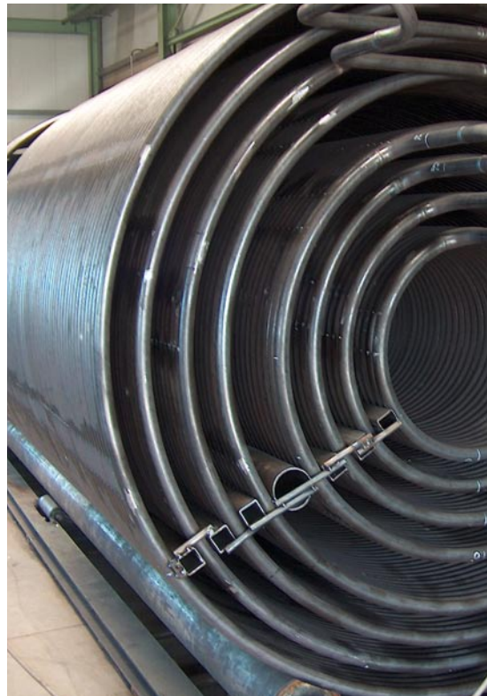
The inside of a condensation preheater
